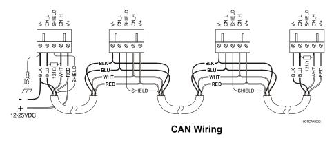
Note: 12 - 24VDC must be supplied to the network.
