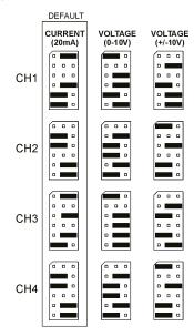
Figure 4. Jumper Array Settings for Each Channel (Channel 1-4) and each mode type.
