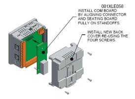
Figure 2 - Installing the COM Board in the XLE
