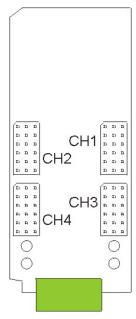
Figure 3. Output Mode Jumper Array locations.
