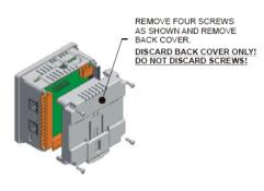
Figure 1 - Removing Back Cover of the XLE
