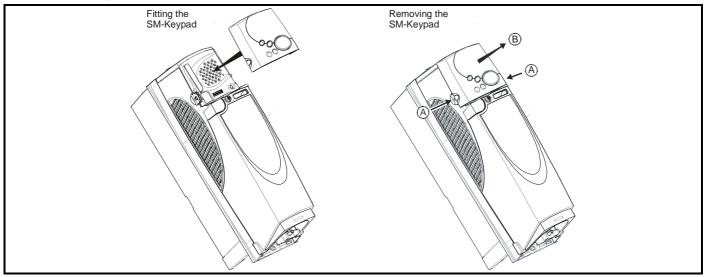
To fit, align the SM-Keypad and press gently in the direction shown until it clicks into position.
